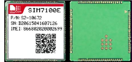
SIMCom presents an ultra compact and reliable wireless module SIM7100E which is based on Qualcomm MDM9215 multiple-mode LTE platform. SIM7100E is a complete multi-band TDD-LTE/FDD-LTE/WCDMA/GSM/GNSS SMT type module designed with very powerful processors integrating application core:Cortex™ A5(550MHz),three QDSP6 cores (Up to 500Mhz), allowing customer to benefit from small dimensions and cost-effective product solutions.
